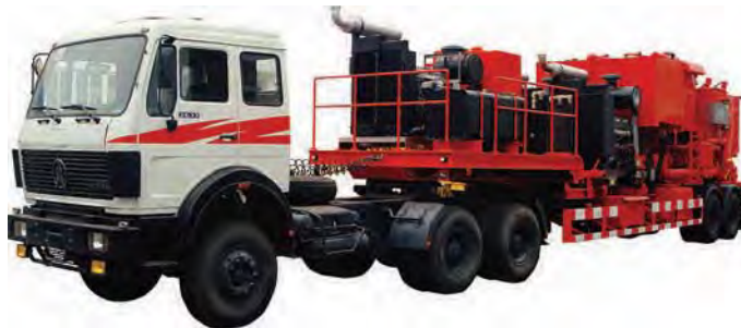
Trailer-Mounted Cementing Unit
